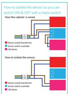
Rewire the cabinet as shown in the diagram above. HiB recommends that all electrical bathroom products should only be fitted by a suitably qualified, Part P registered electrician.
