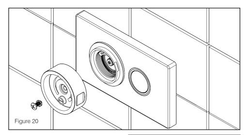
16. On the rear of the handle is a handle stop that sits against the right hand side of the valve temperature stop ring to prevent the handle being rotated past the pre-determined maximum temperature position. Without moving the temperature spindle, position the handle onto the cartridge so that it cannot rotate anti-clockwise.
