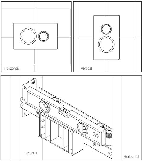
This valve is designed to be installed in stud constructions using timber of a suitable depth as to allow the full installation frame to fit onto the stud (Figure 1). The centre point between the two studs will be the final position of the valve. To ensure successful installation, the frame needs to fit correctly between the two studs without deforming the frame. If necessary use spacers to create the correct fit.
