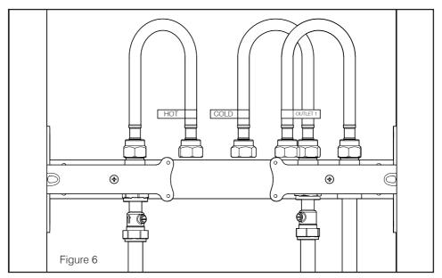
4. Connect the flexible hoses to the manifolds - ensure that each hose has a rubber washer inserted at each end to create a watertight seal. Once connected, label each hose with the corresponding inlet / outlet - this will help easily identify which hose is which during later installation stages.
