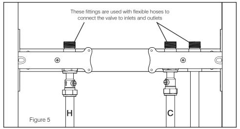
3. With the water inlet supplies installed, install outlet pipework using suitable plumbing fittings. Ensure that there is enough room to route pipework to the chosen outlet location.
