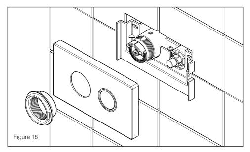
14. Position the cover plate over the valve housing and fix in place with the cover plate fixing nut. Tighten the plate to the wall with the tool provided making sure not to scratch the cover plate. Make sure the cover plate is level and that the button is in line with those on the valve. The cover plate is fitted with an integrated foam seal - it is not necessary to use silicone sealant.
