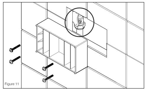
9. Remove the tiling guide, allowing access to the pipework behind the tiled wall. Keep these screws safe as they will be used to mount the valve. From this position the isolation valves should be visible and accessible through the access hole.
