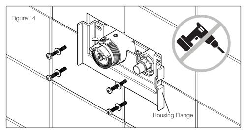
12. Lift the valve and push the hoses back through the access hole, making sure the hoses do not kink (Figure 14). Position the valve flat against the tiles and line up the fixing holes with those on the metal installation frame. Secure the valve to the fixing frame.
