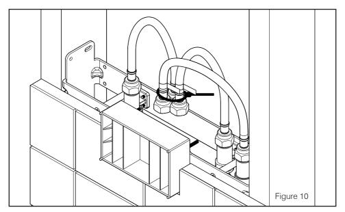
8. Once a hole has been cut in the plasterboard, secure it to the stud. The tile guide should pass through the hole in the plasterboard. Tile up to the edges of the tile guide to ensure the correct size access hole. Failure to do so may mean the cover plate does not form a water-tight seal in later installation stages.
