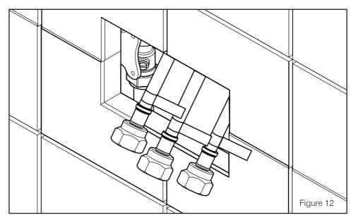
10. Pull the flexible hoses through the access hole in the wall and remove the zip tie.
