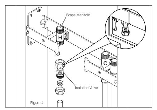
2. Once the frame is installed, remove the plastic tile guide. Install the supply pipework to the isolation valve and the brass manifolds. The hot water feed should be installed into the left hand manifold and the cold water feed to the right hand manifold. Ensure the isolation valves are mounted so that they will be visible and accessible for later stages (Figure 4).
