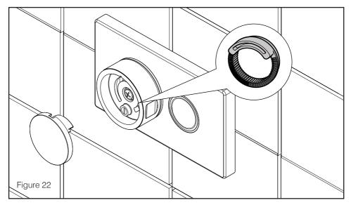
18. With the handle installed, the centre dial can be pushed into place. The dial has a tab that fits into the temperature stop ring via a gap in the handle. To remove the dial for maintenance, line up the notch in the centre dial with the notch on the handle and use a small screwdriver to separate the two parts.
