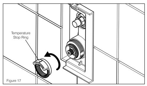
The temperature stop ring is installed onto the temperature cartridge fixing nut on the valve. This prevents the maximum temperature from being exceeded when in use. For vertical installations the temperature stop ring needs to be removed and rotated 90 degrees as shown (Figure 17)
