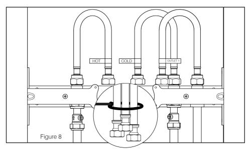
6. Once satisfied that there are no leaks, turn the water supply off and disconnect the valve from the flexible hoses. Before installing plasterboard and tiles, use the zip tie provided to tie the ends of the hoses together to make them easier to access later.
