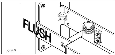
1. Position the installation frame between the two studs or noggins at a suitable height for its final installation position. The front of the frame and the front of the timber stud should be flush (Figure 3). Use a spirit level placed on the tiling guide to make sure the installation frame is level both front to back and left to right. Once level remove the tile guide and keep the fixing screws safe for later steps.
