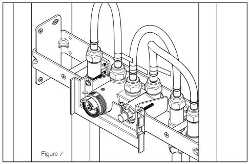
5. At this point it is critical that leak tests are performed. Connect the valve body to the flexible hoses - the hot and cold inlets are marked with red and blue paint on the valve. Turn on the water supply and test the system for leaks. Push the button for the outlet and check all connections are fully sealed.
