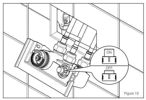
11. Working from left to right, using the labels as a guide, connect the hoses to the valve. Ensure the hose from the hot supply is connected to the inlet marked hot on the valve. Do the same for the cold supply. Ensuring the outlet button is in the 'OFF' position (Figure 13), turn the water supply back on at the isolation valve. Do not overtighten the hoses as this may damage the rubber washers.
