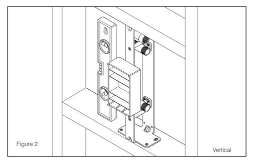
For vertical installations, timber noggins should be installed between studwork to allow for the frame to be fixed vertically. (Figure 2)
