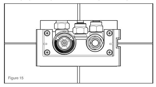
13. When secured in place, the fixing nuts of the flexible hoses will be visible above the valve housing. This will allow the connections to be checked for leaks and for the hoses to be tightened slightly, if necessary, without removing the entire valve.
