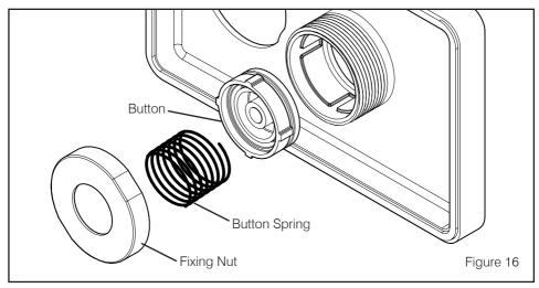
Remove the brass fixing nut from the back of the cover plate, as shown above. This will allow the etched button and spring to be removed. Rotate the button 90 degrees and reassemble to the cover plate. (Figure 16). There are four slots which ensure the button is located correctly. With the spring assembled inside the channel on the back of the button, reassemble the brass fixing nut.
