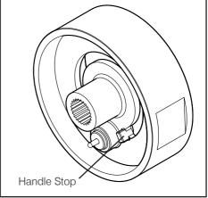
17. Once installed, the handle should click as it rotates. This click can be adjusted to give more feedback when in use.
