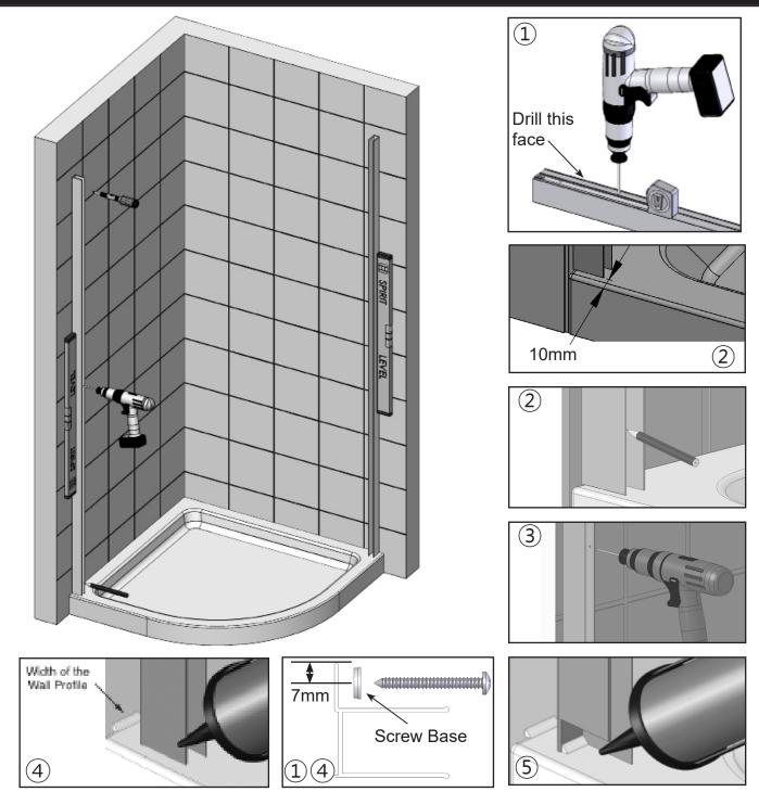
1. On both wall profiles drill three 4.5mm holes through the lip. Place them 7mm in from the edge and approximately 100mm from each end and the other positioned in the centre.
