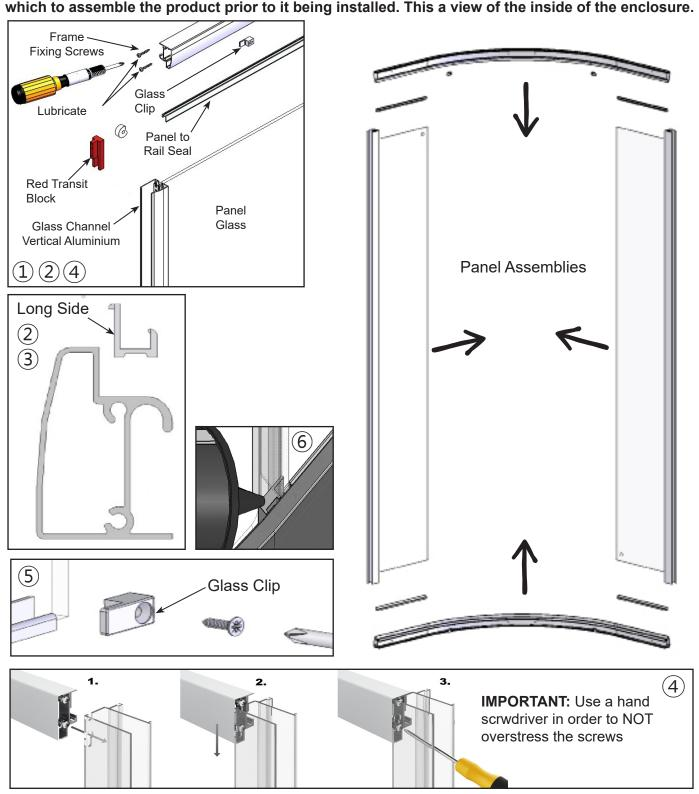
NOTE: This part of the installation requires 2 people and a clear area in front of the shower tray in which to assemble the product prior to it being installed. This a view of the inside of the enclosure.
