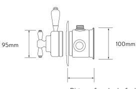
Distance from back of valve to finished wall surface (includes 10mm allowance for tiles) Min. 68mm Max. 82mm
