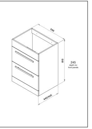
Dimensions (measurements in mm)
