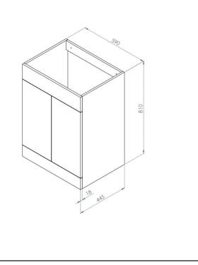
Dimensions (measurements in mm)
