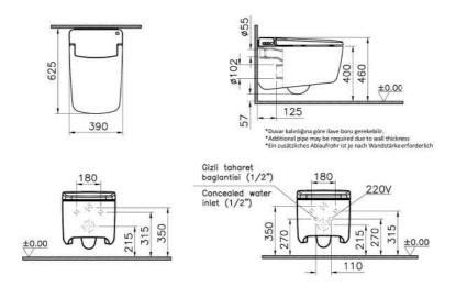
All drawings contain the necessary measurements which are subject to standard tolerances. For exact measurements, in particular for customized installation scenarios, it can only be taken from the finished ceramic product.
