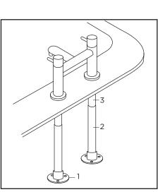
Place the tap tails through the bath platform and screw on the tap connector (4) tightly.
