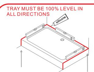
Ensure the shower tray is level in all directions and is properly sealed to the wall. The wall must be tiled down to the top edge of the tray. **Do not angle out bottom tile**.
