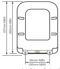
max/min fixing adjustment
