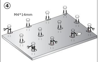
Screw the feet in position with the screws provided. Ensure that the foot that has two panel fixing rods attached, is placed in the corner where the panels will meet.
