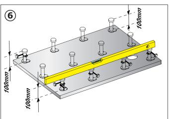
When all of the feet have been fitted, the feet in the corner positions should be adjusted to 100mm.
