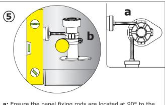
**a:** Ensure the panel fixing rods are located at 90° to the edge of the tray as shown above.
