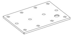
Turn the tray over and use the cardboard packaging as a protective mat. Note the circles that have been marked to indicate feet position. The symbol  $\bigoplus$  indicates where you should fix the feet with the panel fixing rod, but for the symbol  $\bigoplus$  you will only use five of these positions and the other three would be supplemented with the feet without the panel fixing rod.
