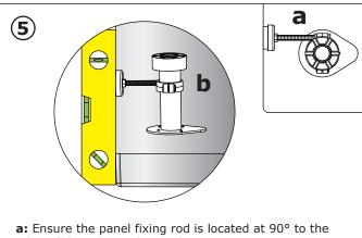
**a:** Ensure the panel fixing rod is located at 90° to the edge of the tray as shown above.
