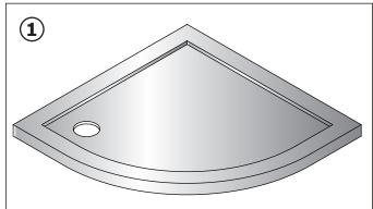
Remove protective plastic film from the areas near the waste and those sides of the tray which will be against a wall.
