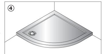
Fit the shower tray waste. Ensure the two side edges are flat to the wall. Place the shower tray onto the cement bed and apply gentle pressure with the palm of the hand to bed the tray into position.
