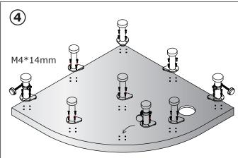
Screw the feet in position with the screws provided. Ensure that the feet that have panel fixing rod attached, are placed around the curved edge where the panel will meet.
