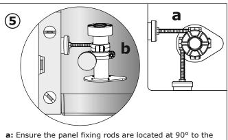
a: Ensure the panel fixing rods are located at 90° to the edge of the tray as shown above.
