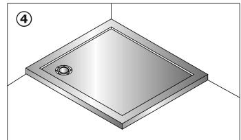
Fit the shower tray waste. Ensure the two side edges are flat to the wall. Place the shower tray onto the cement bed and apply gentle pressure with the palm of the hand to bed the tray into position.
