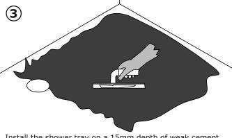
Install the shower tray on a 15mm depth of weak cement mix (sand/cement ratio 5:1). Tile adhesive can be used as an alternate to sand or cement.
