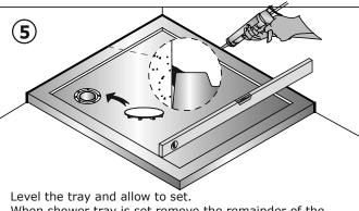
When shower tray is set remove the remainder of the protective plastic film and connect the waste pipe and check for leakage.
