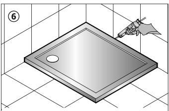
Tile and seal joints with an anti fungal silicone sealant and allow to set.
