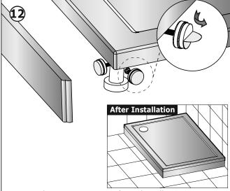
Remove the protective cover from the adhesive tape. First fix the rebated panel pushing it firmly on to the adhesive pads. Then fix the remaining panel in the same manner.
