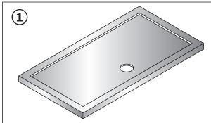
Remove protective plastic film from the areas near the waste and those sides of the tray which will be against a wall.
