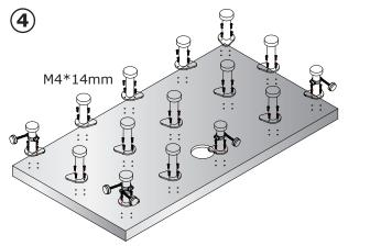
Screw the feet in position with the screws provided. Ensure that the foot that has two panel fixing rods attached, is placed in the corner where the panels will meet.
