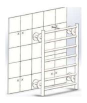
Use a measuring tape to measure the distance between the center points of each wall bracket tube, and mark the installation holes by pencil.
