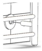
Connect the core wire from the leg to the power wire inside the wall
