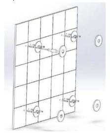
Insert long screw through mounting seat , then screw into the plastic wall anthor with a screw driver. And put the decorative cap against the mounting seat
