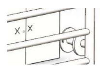
Be sure to drill a hole for the core cable going from the leg to the wall on the right lower mounting leg.
