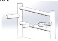
Fix 3 mounting single hole tubes to the threaded holes on the vertical bar, Screw down the mounting screw with a screwdriver.
