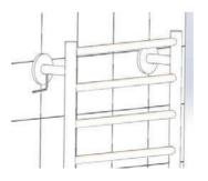
Install the hex screws into the hole of all the tubes using the allen wrench and fix the towel warmer tube onto the mounting bracket.
