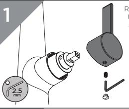
Remove cap. Undo grub screw and remove handle.
