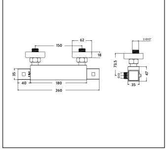
Dimensions (measurements in mm)
