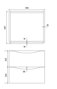
Dimensions (measurements in mm)
