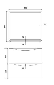
Dimensions (measurements in mm)
