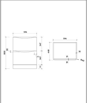
Dimensions (measurements in mm)
