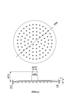
Dimensions (measurements in mm)
