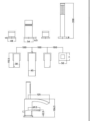
Dimensions (measurements in mm)
