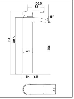
Dimensions (measurements in mm)
