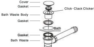
From the underside of the bath push the gasket onto the waste housing. From inside the bath place the plug hole in position on the gasket and screw the waste body into the waste housing.
