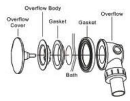
Push the gasket onto the overflow housing and hold the unit inposition from the outside of the bath. From the inside of the bath place the gasket and overflow body over the overflow hole. Finally screw on the overflow cover.
