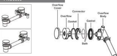
Push the gasket onto the overflow housing and hold the unit in position from the outside of the bath. Prepare the overflow assembly by pushing gasket into the connector piece, then push the overflow filler onto the overflow body. Finally, screw the overflow cover into the overflow body ensuring that a watertight seal is made at the overflow. If the hole is to small, snap off one of the lugs with a pair of long nose pliers.
