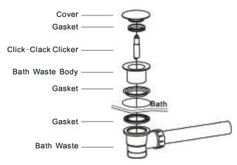
From the underside of the bath push the gasket onto the waste housing. From inside the bath place the plug hole in position on the gasket and screw the waste body into the waste housing.
