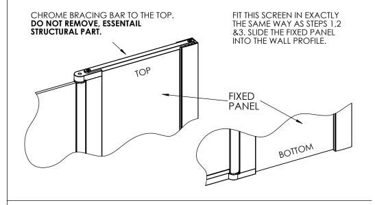
4. SILICONE AS BELOW ---- ALLOW 24 HOURS TO DRY BEFORE USING.
