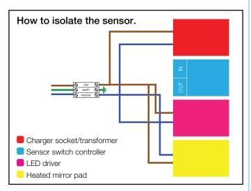
Rewire the mirror as shown in the diagram above. HiB recommends that all electrical bathroom products should only be fitted by a suitably qualified, Part P registered electrician.
