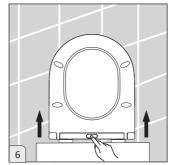
6.To remove the seat press the quick release button and lift off.
