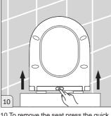
10.To remove the seat press the quick release button and lift off.
