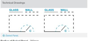
Radius of Swivel Panel - 290mm Recommended opening min 500mm
