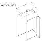
Supplied with high level vertical post. Post supplied 3 metre maximum length (designed to be adapted to size). Recommended opening min 500mm.
