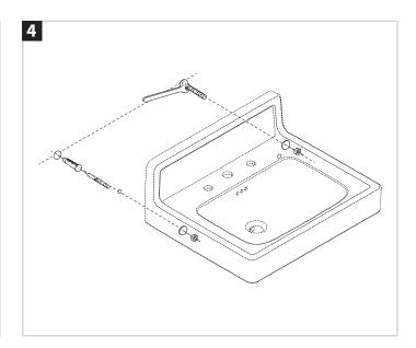
The basin must always be fixed to the wall using appropriate wall fixings.
