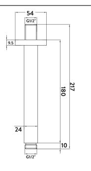
Dimensions (measurements in mm)
