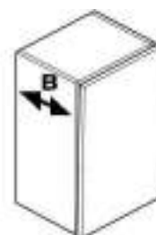
B- Lateral Loosen screw 'B'. Adjust door and retighten screw.
