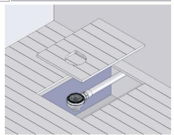
Lift the floorboards from the centreline of joists to plumb the waste unit into the correct position - refer to waste unit instructions.
