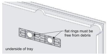
On underside of tray, ensure the flat ring around the relevant waste hole (or both holes if fitting two wastes) are free from debris. Wipe clean if necessary.
