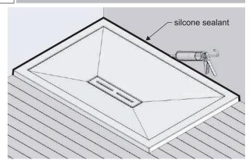
Before tiling/panelling walls, any gap between the tray and walls must be filled with silicone sealant flush to top of tray.
