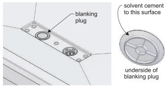
Apply a full continuous bead of solvent weld cement (not supplied) to underside flange of blanking plug.
