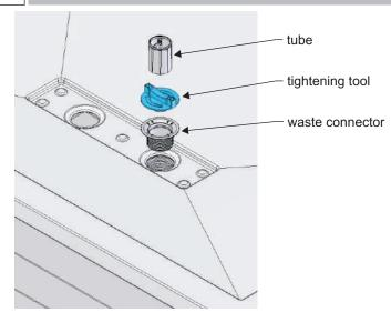
Apply silicone sealant to underside flange of waste connector and screw fix into waste unit, fully tighten using the blue tightening tool supplied, as shown, then fit tube into connector. Wipe away any surplus sealant with a clean, damp cloth.
