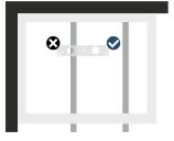
Where joists run parallel to the width of the tray, at least one hole will always be clear.
