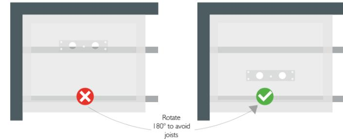
Where joists run parallel to the length of the tray and both holes are obstructed, simply turn the tray 180°. The unique offset position will ensure both will be free.
