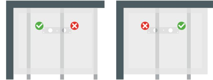
Where joists run parallel to the width of the tray at least one hole will always be clear.
