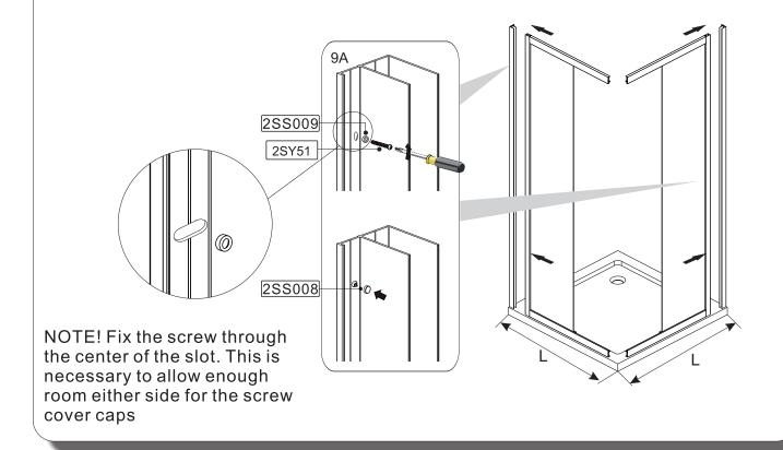
10A.Slide both corner brackets fully onto each end of the profiles and fix to the frame with screws and cover clips.
