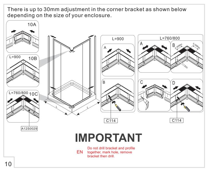
After your corner bracket has been fixed you can square your enclosure on the tray and fix the wall profiles to the upright profiles as shown below.
