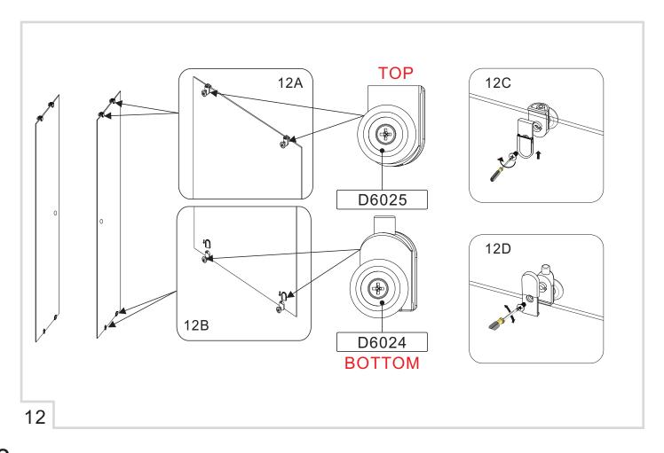
To fit your door panel firstly hange the top roller to support the weight of the glass panel. You can then leave your door panel hang making it easier to release your easy clean roller into the bottom track
