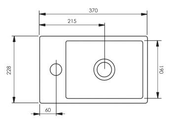
DIAGRAMS NOT TO SCALE | ALL DIMENSIONS IN MM TOLERANCE OF  $\pm$  5mm  $\,$  ALL PRODUCTS CONFORM TO BRITISH STANDARDS  $\,$
