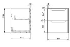
Dimensions (measurements in mm)
