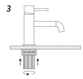
Slide Easy Fit Fixture onto \*\*tap end\*\* until top of the fixture touches the basin.
