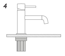
Push and twist clockwise to tighten. The gap will begin to close.
