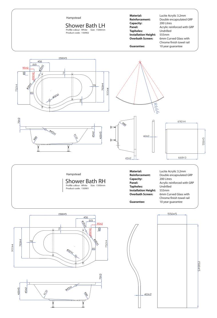
Hampstead Shower Bath LH Profile colour: White Size: 1700mm Product code: 170902 Material: Capacity: Reinforcement: Panel: Tapholes: Installation Height: Overbath Screen: Lucite Acrylic 3.2mm 220 Litres Double encapsulated GRP Acrylic reinforced with GRP Undrilled 555mm 6mm Curved Glass with Chrome finish towel rail 10 year guarantee
