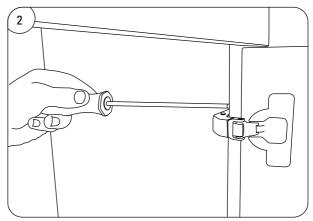
If the delivered configuration isn't suitable remove door from unit using a suitable tool.
