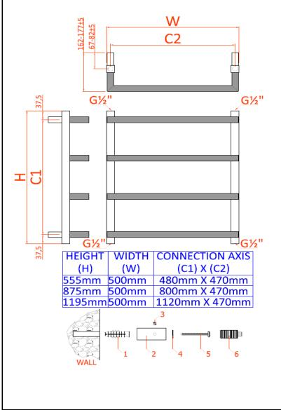
The radiator should not be mounted closer than 50mm below any overhanging surface (i.ei shelf) and no lower than 100mm from the floor. Transfer the bracket drill position measurements to the wall.
