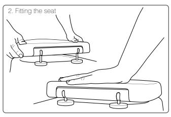
Align and insert the pins into the seat hinge sockets and firmly press down until you hear them 'click' into position.
