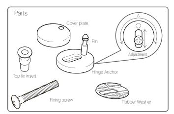
Maximum adjustment of the pin position is achieved by rotating the hinge anchor around the screw (adjustment A above). Further fine adjustment of the pin position can be achieved by sliding the screw in the slot (adjustment B).
