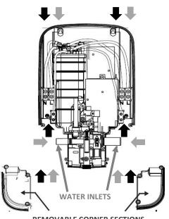
REMOVABLE CORNER SECTIONS FOR EASE OF TOOL ACCESS
