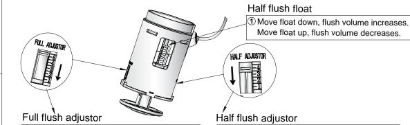
2 Move adjustor down, flush volume increases. Move float up, flush volume decreases.
