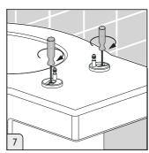
7.Fully tighten the fixings.
