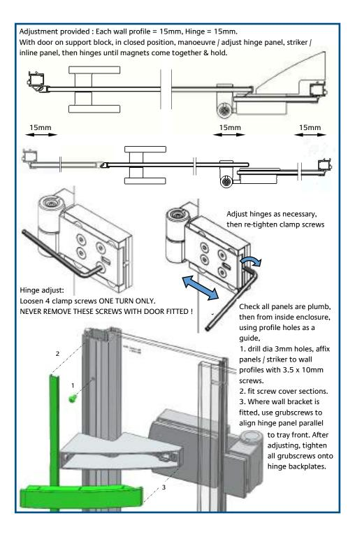
Support block may now be removed. Open / close the door & re adjust hinges to fine tune the door magnets. Visually check both hinges for riser clearance, if one shows clearance, turn its take up screw until white plastic castellated faces are in full contact when the door is closed.
