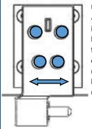
Undo / remove the 4 clamp screws indicated, flip the hinge bracket over, fit & re tighten the clamp screws (on completion, both pins will be upright). Apply continuous bead of clear silicone to inside of bottom channel, then carefully push bottom trim upto vertical profile & then onto glass bottom edge. A mallet, or hammer & wood block may be used. Take care to avoid bending the trim !
