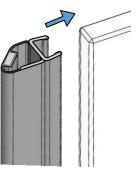
Magnetic Seals : Align seal end with top of glass, press fit onto door or panel edge.
