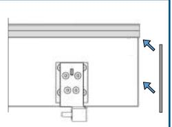
Hinge panel sub assy's are supplied with hinge pins facing one another. Before use, offer panel to hinge side wall, reverse the top hinge, & fit bottom channel:
