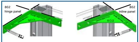
3. BEFORE DRILLING : Assemble glass brackets onto panels & tighten clamp screws. Position brackets as close to panel ends as possible. Model 803 : site the bracing bar tee clamp 10mm from door glass edge\*\*\* ! Then offer entire bracing bar into place to check that wall bracket locations are correct.
