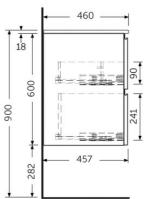
Dimensions: All dimensions in mm tolerance ±5% for below 200mm and ±3% for above 200mm.
