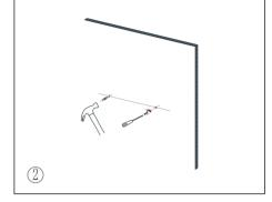
Insert the wall plug and mounting screw into the wall.
