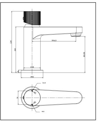
Dimensions (Measurements in mm)
